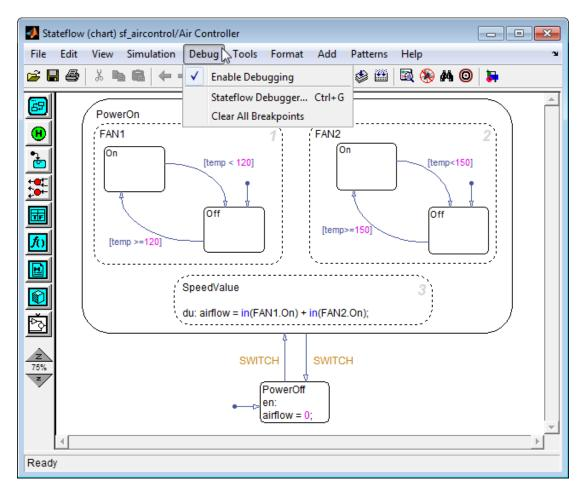
This enhancement enables you to focus on debugging a single chart, instead of having to debug all charts in the model. For details, see How to Enable Debugging for Charts in the Stateflow User's Guide.
